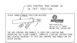
NOTE: Handle cannot be turned from "PILOT" to "OFF" unless handle is pushed in slightly. Do not force.
